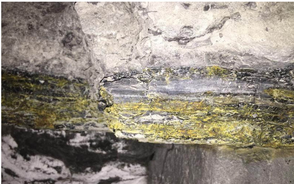
A seam hosting 2% uranium and high-grade vanadium (the black rock) at Western Uranium's past-producing Sunday mine in Colorado. Credit: Western Uranium.
